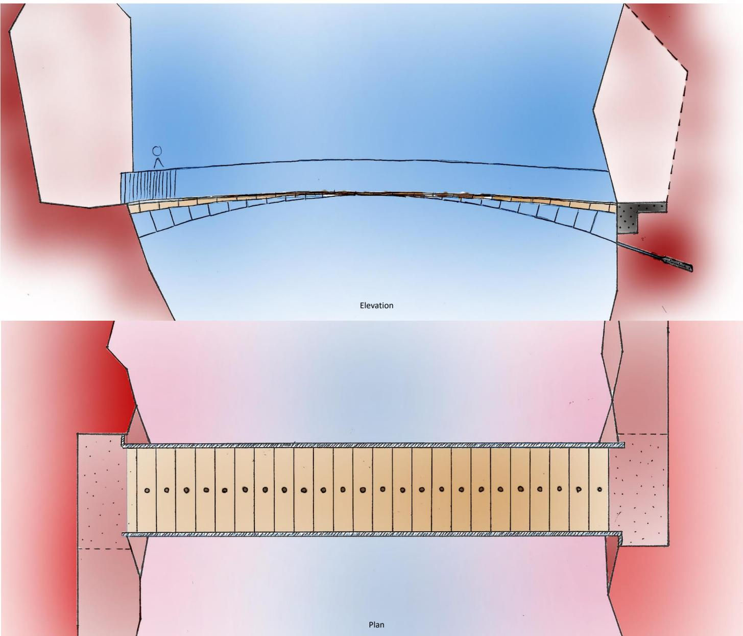
**Structural system:** A walk on arch bridge formed from UHPC blocks, a cable below, and stays connecting the two. The arch and cable have foundations in the cliff faces on each side of the bridge.
