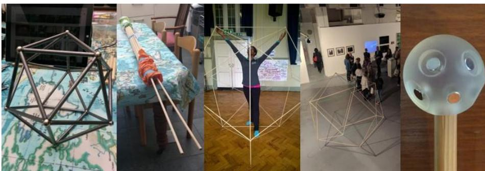
*Figures 1a-1e: Early 'brittle' model with spherical magnetic nodes and steel rods; Prototype ready for transport; First prototype in use; Second prototype; experimental resin node (nodes are wooden on prototypes)*
